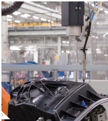
1 Crash beams without (left) and with SikaPower® (right) 2 Car body in robotic cell 3 SikaPower® application at shock tower
