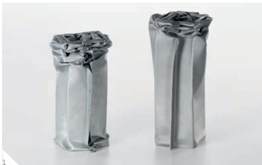
1 Crash beams without (left) and with SikaPower® (right) 2 Car body in robotic cell 3 SikaPower® application at shock tower
