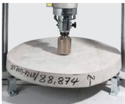
Ensaio de painel circular: ASTM C 1550
